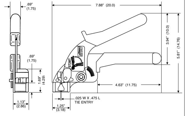
NOTES, UNLESS OTHERWISE SPECIFIED: PANDUIT TOOL NUMBER ST2MT IS USED TO INSTALL ALL STANDARD, LIGHT-HEAVY, HEAVY AND EXTRA-HEAVY CROSS SECTION PAN-STEEL TYPE MLT TIES, TYPE MLTC COATED TIES AND TYPE MLTDH DOUBLE WRAPPED TIES.
